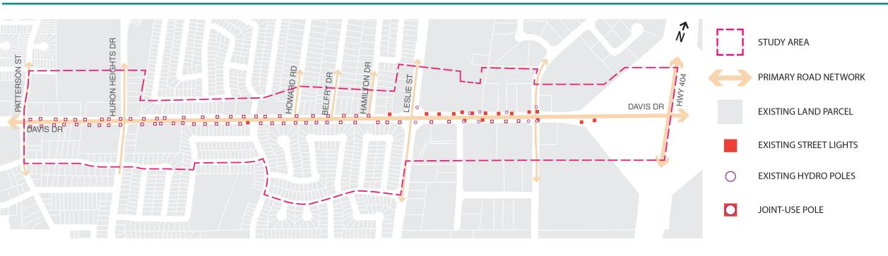
The average distance between light standards is 45 metres oncentre. The average spacing of hydro poles is 45 metres oncentre.
